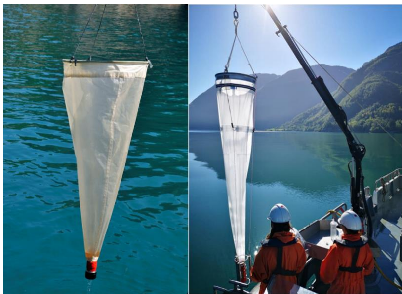
Figure 15. The plankton net used for the large volume haul samples from the ØKOKYST program.
