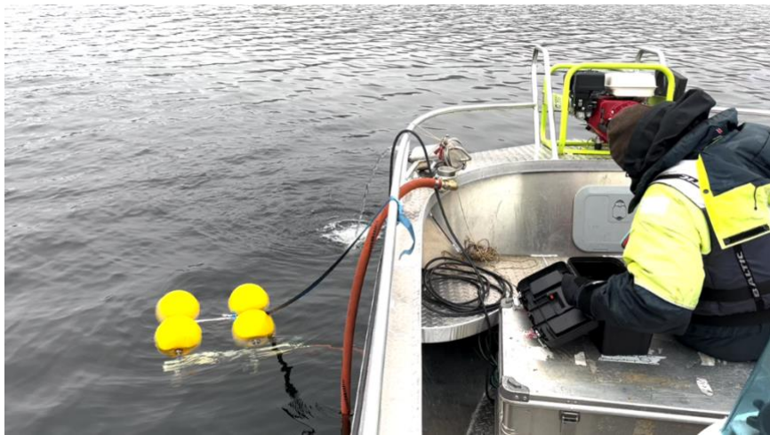
Figure 16. Deployment of the large volume microplastic pump and filter system by the Urbanfjord and Milfersk program.
